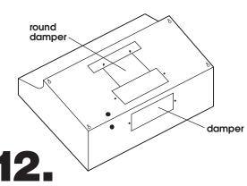
Attach rectangular damper to selected rectangular vent opening. If damper is attached to back of range hood, be sure damper hinge is toward the top. For round vented installations, use round damper in vent to prevent air from flowing back into ventwork. If wall or roof cap has a damper, remove damper blade from range hood.
